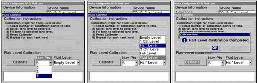
**Num Pts menu with 5-point calibration selected (left). Half level selected on Fluid Level menu (center). Calibration completed window (right).**
