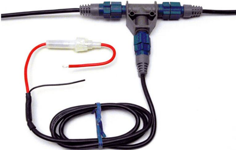
**OEM factory installations typically use a Power Node similar to this to supply power to the network bus. The red and black leads are connected to a switched power source, allowing the user to turn off power to the bus.**
