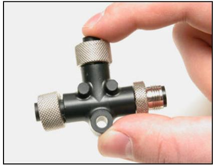
**The T connector with blue connectors (left). DeviceNet Micro-C connector (right) used in some NMEA-2000 buses.**
