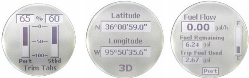
Trim Tabs page (left), GPS Module page (center) and Fuel Manager Page (right).
