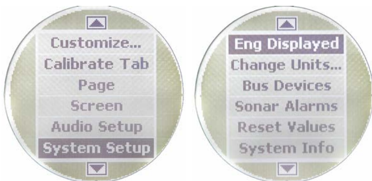
Basic menu with System Setup highlighted (left). System Setup menu (right) with Engine Displayed selected.
