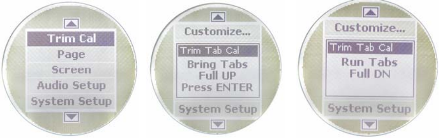
Trim Tabs menu (left). When calibrating Trim Tabs, the Full Up message (center) appears first. It is followed by the Run Tabs Full Down message (right).
